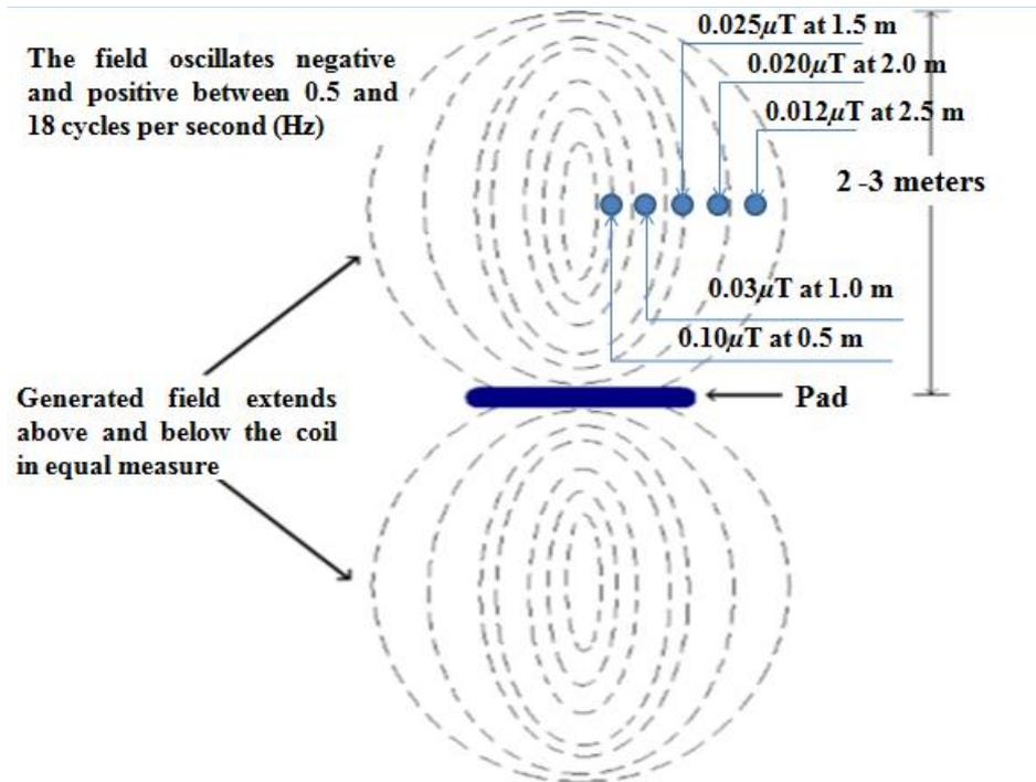
Figure 1 The approximate shape of the predominant enclosed electromagnetic fields when the frequency is at 12Hz
