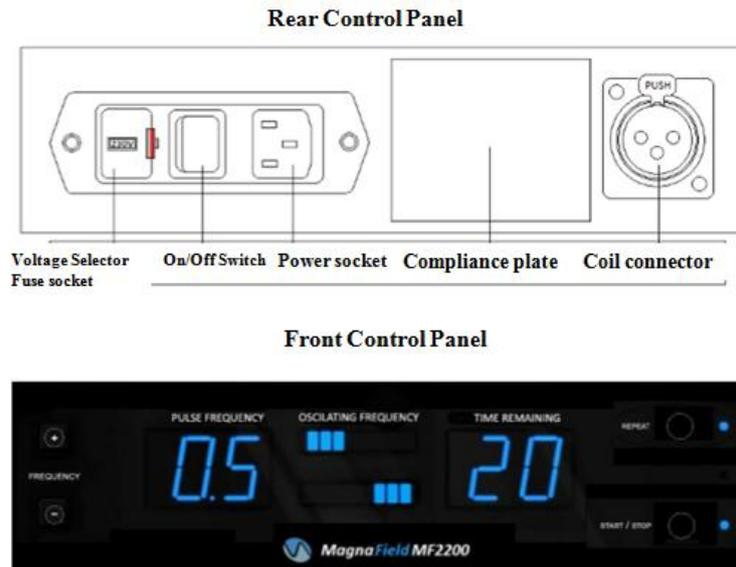
Figure 2 The front and rear control panels
